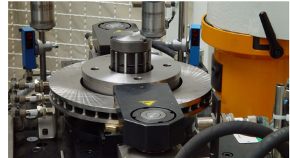
Facing chuck and multi-blade mandrel
