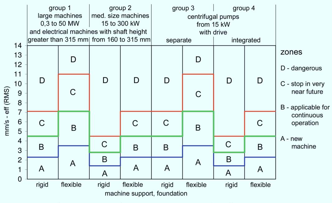
Zones for assessment of vibration severity in mm/s - eff evaluated for machines installed at site (acc. ISO 10816 - 3)
